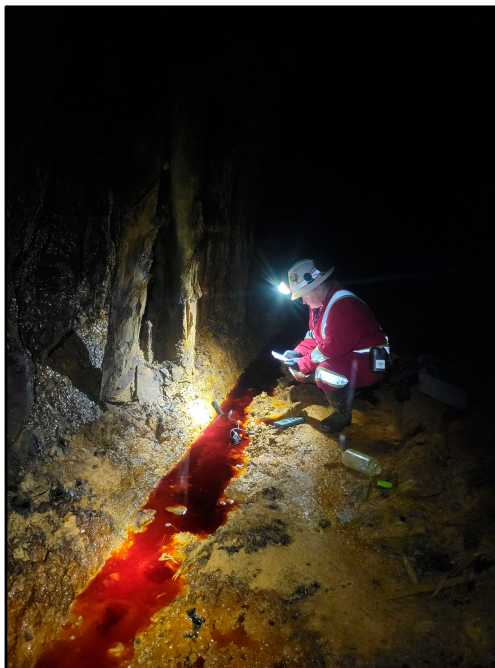
Figure 7. Sampling of mine water at the pyritic zone site 5GH2, Bunker Hill Mine (Pictured: Morgan Hill, Bunker Hill Mining Corporation).
